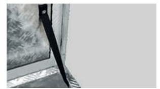
Anti-opening strap with rubber insulation. Modelos: R70, R120, R234.
