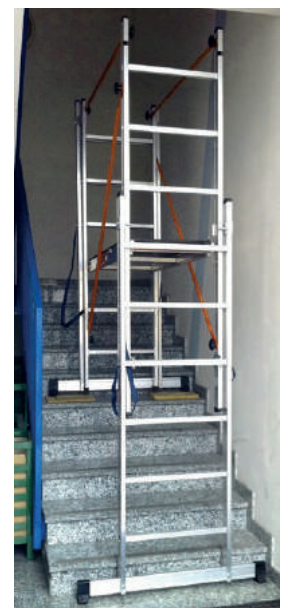
Possibility to work in the stairs.
